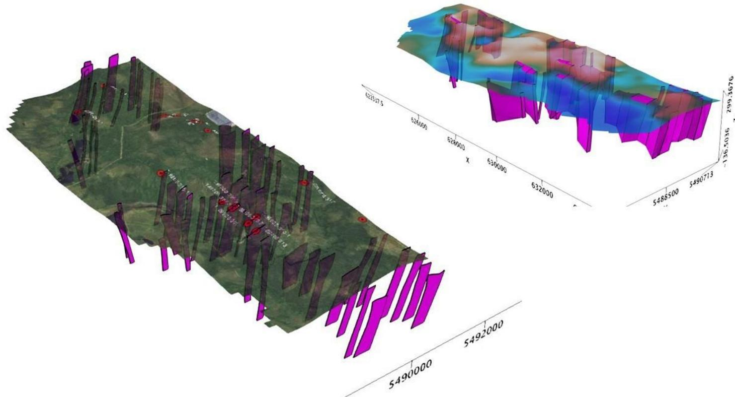
Figure 17: Gold Trends Interpretation Based on Drilling Data, Magnetics, and VLF Signatures.
